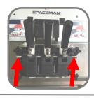
Adjustment screws below draw handles control dispensing speed.
