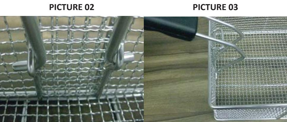
2) Press the upper portion of the hoop wire against the upper housing of the basket until the basket is well fit, as shown in pictures N°03 and N°04.
