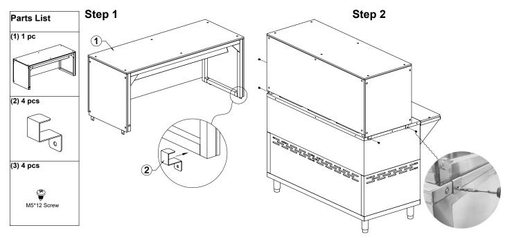
Step 1: Attach the (4) brackets to the bottom tube of the sneeze guard.
