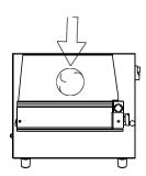
The small dough (20-500g) which have ferment previously (at least 4 to 6 hours), squash the sides slightly and put some dry flour on it so it can easily go through the upper rollers.
