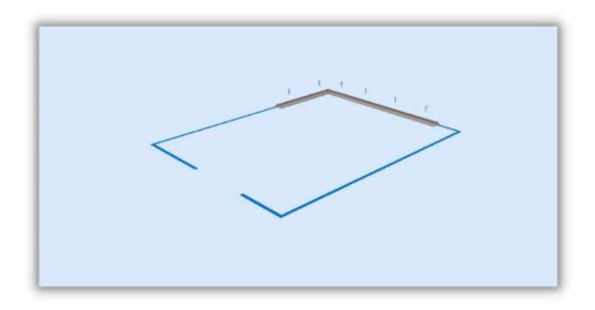
**Step 2**: Start panel assembly by inserting the rear corner wall panel (CWNF1 or CWNF3) into the vinyl screed as per your assembly drawing.
