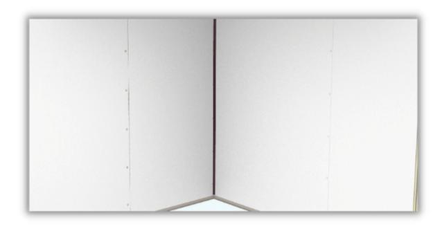
2. Snap the white sanitary profiles into the black seam tracks.
