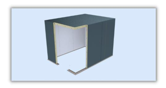
**Step 10**: Attach and fasten the door header panel to the door frame panel.
