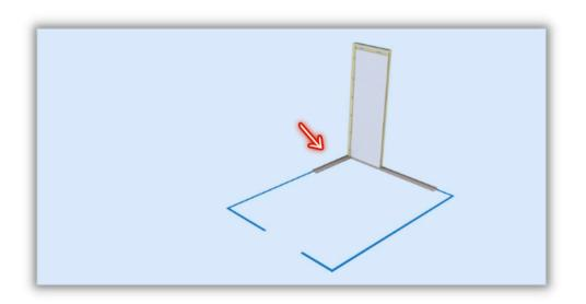
**Step 3**: Work your way toward the front of your box by adding vinyl screeds and attaching the wall panel adjacent and perpendicular to the rear corner panel as per your assembly drawing (WNF15, WNF30, or WNF45). Fasten the wall panels to each other.
