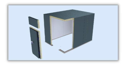
**Step 11**: Attach the fully-assembled door panel to the wall and ceiling panels as per your assembly drawing.
