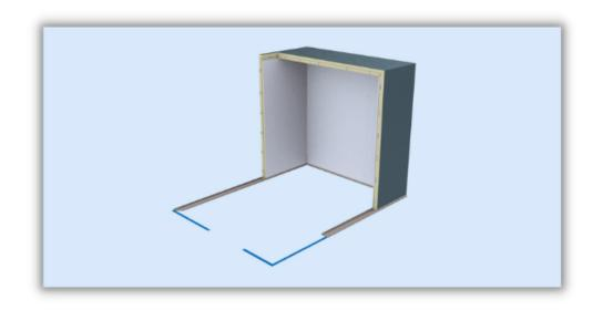
**Step 7**: Continue assembling wall panel(s) on one side of the box as per your assembly drawing. Fasten the wall panels to each other.
