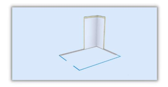
**Step 4**: Continue assembling wall panels and vinyl screeds in the direction of the other rear corner as per your assembly drawing and the renderings below. This provides stability as you build your box.
