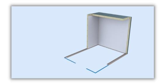
**Step 6**: Attach the wall panel serving as an end cap to the ceiling panel (WNF or CWNF on your assembly drawing) to the wall and ceiling panels.
