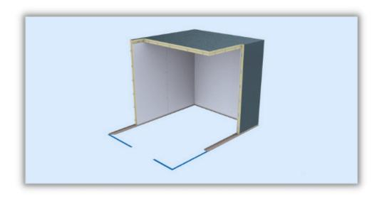
**Step 9**: Continue working your way to the front of the box by assembling vinyl screeds, wall panels, and ceiling panels on each side of the box as per your assembly drawing and the following renderings:
