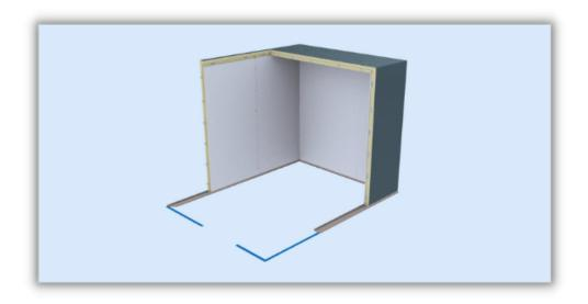
**Step 8**: Attach the next ceiling panel (as per your assembly drawing) to the rear ceiling panel and the wall panel(s) you assembled in the previous step.
