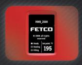
Touchscreen interface for easy access to temperature controls, metrics and diagnostic screens.
