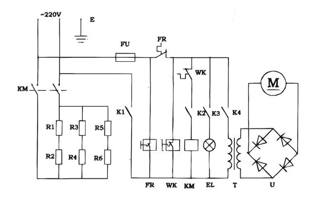
R1~R6—ELECTRIC HEATING TUBE K1—STOPPING SWITCH K2—HEATING SWITCH K3—LIGHTING SWITCH K4—ROTATING SWITCH WK—TEMPERATURE CONTROLLER INSTRUMENT KM—CONTACTOR
