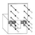
**4.** Remove original support brackets (x2) and back plate assembly from range. Discard original support brackets (x2).
