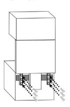
**14.** Attach heat shelf to backsplash using **B** bolts (x2), flat washers (x2), and spring washers (x2).
