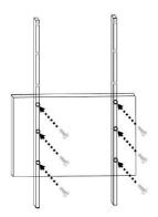
7. Remove A bolts (x8), flat washers (x8), and spring washers (x8) from back of salamander (specified in below diagram). Keep A bolts (x4), flat washers (x4), and spring washers (x4) for step 8.
