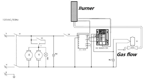
HL1-----Power indicator HL3-----Ignition indicator S2-----COOK/COOL switch S4-----Gas ignition switch IC2-----Ignition module M1/M2------Motor HL2------Motor indicator S1-----Power on/off switch S3-----Micro switch IC1-----Digital thermostat YV-----Solenoid valve
