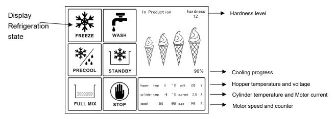
The refrigeration state will blink on the screen during REFRIEGRATION is ON.
