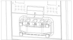
Install the draw valves. Slide the o-rings into the grooves on the draw valve and lubricate.
