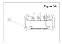
The draw handle can be adjusted to provide a flow rate of 5 to 7-1/2oz of product per 10 seconds. To increase the flow rate, turn the screw clockwise. Turn the screw counterclockwise to decrease the flow rate. Figure 5-9
