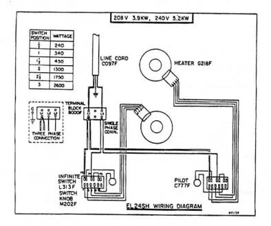
NOTE: A separate circuit should be supplied for each of these stoves with a matched circuit breaker or fuse. Check local codes for compliance in installation.
