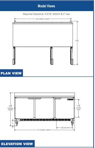
\*NOTE: Remote units are field wired and come with 6" legs. Refrigerant must be specified at time of order.
