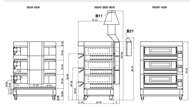
NOTE: The dimensions indicated in the views are in inches. B11 DIRECT VENTILATION (ø 9 27/32"). B21 UNDER VENTILATION HOOD
